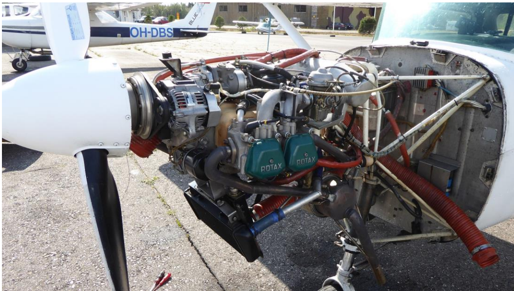
PICTURE 3. Rotax 912S installed on a Cessna 150 (Atol Avion)
