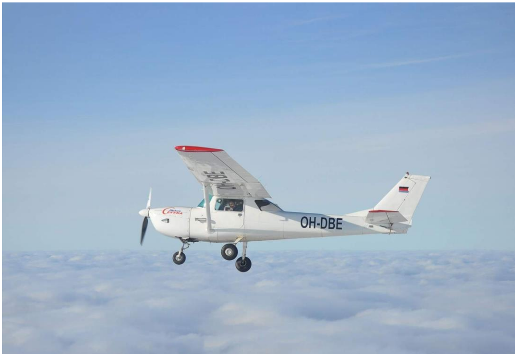
PICTURE 2. Rotax-modified Cessna F150-K (Atol Avion)
