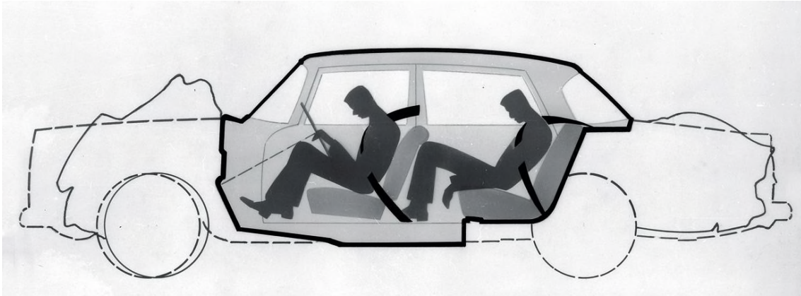
Figure 1. Crumble zone technology with the rigid body (Mercedes – Benz)
