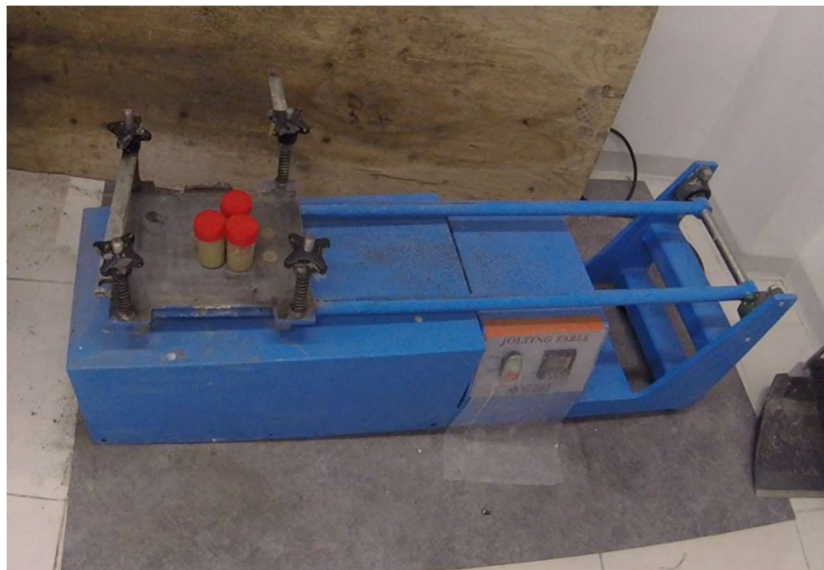
Figure 12 Jolting table for removing air bubbles (Kohvakka, 2020)
