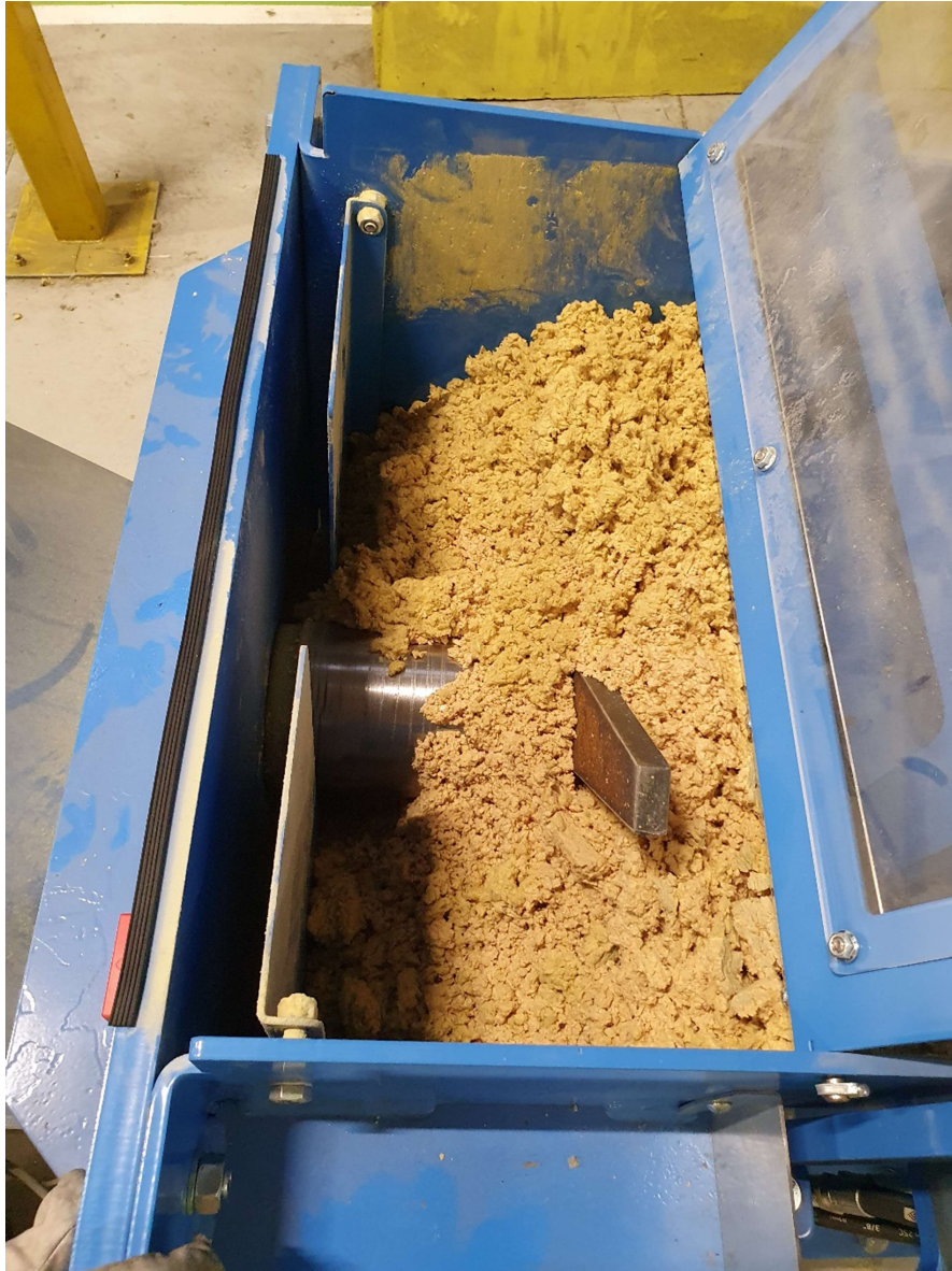
Figure 30 The material has been pushed through the machine, dissipating the plug (Kohvakka, 2020)
