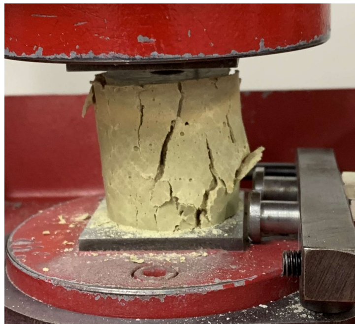
Figure 29 Geopolymer sample with a splitting failure mode (Hukkila, 2020)
