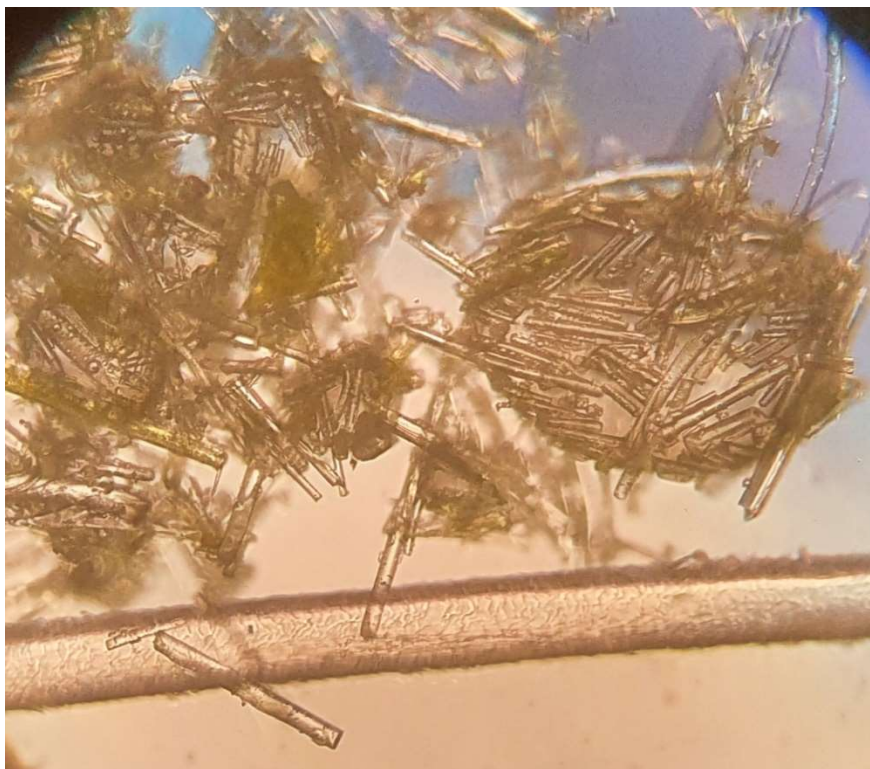
Figure 20 Microscope image of milled GW sample, magnification 140x, human hair as reference (Kohvakka, 2020)
