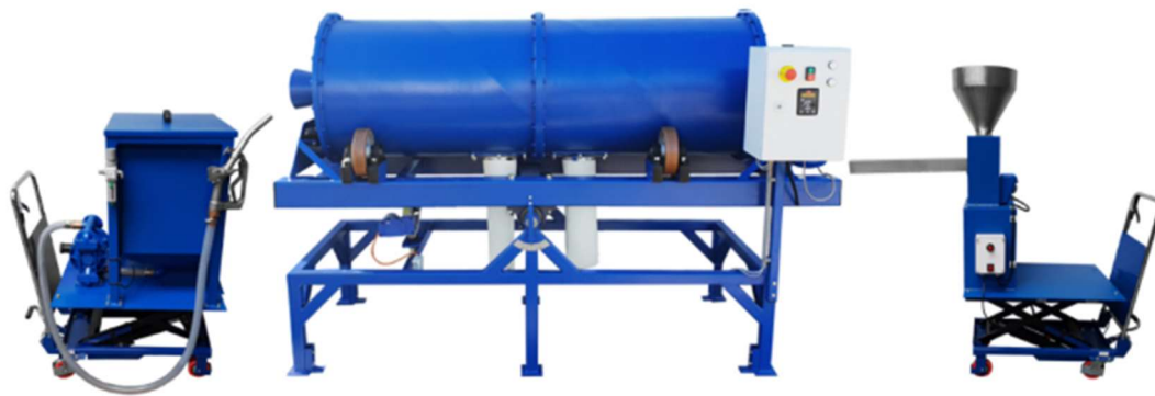
Figure 4 Continuous ball mill for pilot scale milling (Laarmann Group, 2018)
