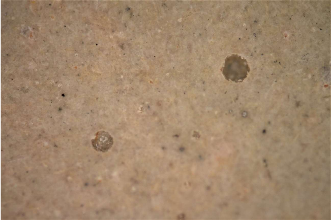
Figure 36 Geopolymer sample, holes left by air bubbles (Kohvakka, 2020)
