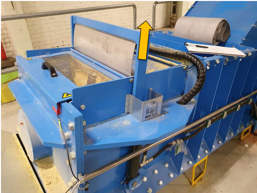
Figure 31 The pressure yoke has lifted, letting material flow through (Kohvakka, 2020)
