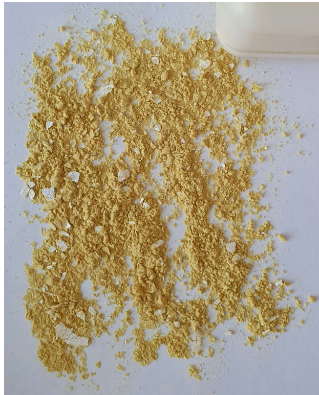
Figure 19 Milled sample before sieving, acoustic panel coating fragments are visible (Kohvakka, 2020)
