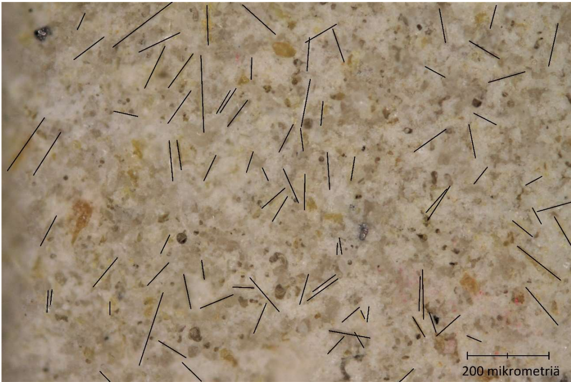
Figure 27 Remaining fibers after hydrolysis highlighted in black, reference bar 200 \mu\text{m} (Kohvakka, 2020)
