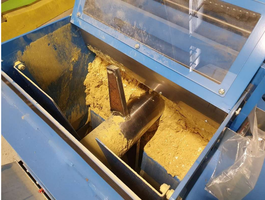
Figure 9 Outlet chamber, showing finely milled GW exiting the mill (Kohvakka, 2020)
