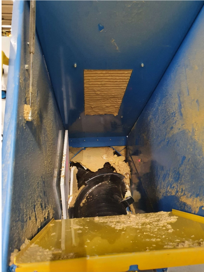
Figure 8 Mil-Tek IC60 inlet chute and the milling screw (Kohvakka, 2020)
