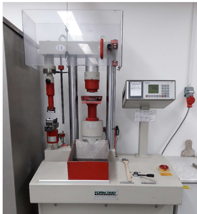
Figure 18 Form+Test Digimaxx C-20 compressive testing machine (Hukkila, 2020)
