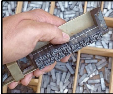
Picture 5 Hand setting with composing stick, from left to right, upside down.
