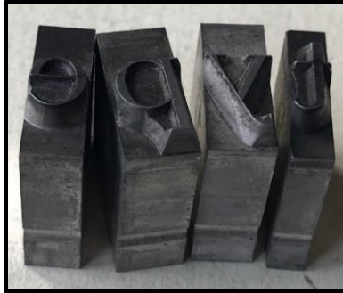
Picture 4 Types, with face on the top, “the nick” (the groove of the bottom of the type) is for knowing which way the type should be set. The “type high” in Europe is 23.56 mm (except in the UK)
