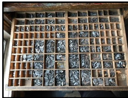
Picture 6 Swedish version of a case, a wooden tray with compartments for storage of type. The bigger compartments are for the letters you use most often. In the English version it looks different because you use other letters more often.
