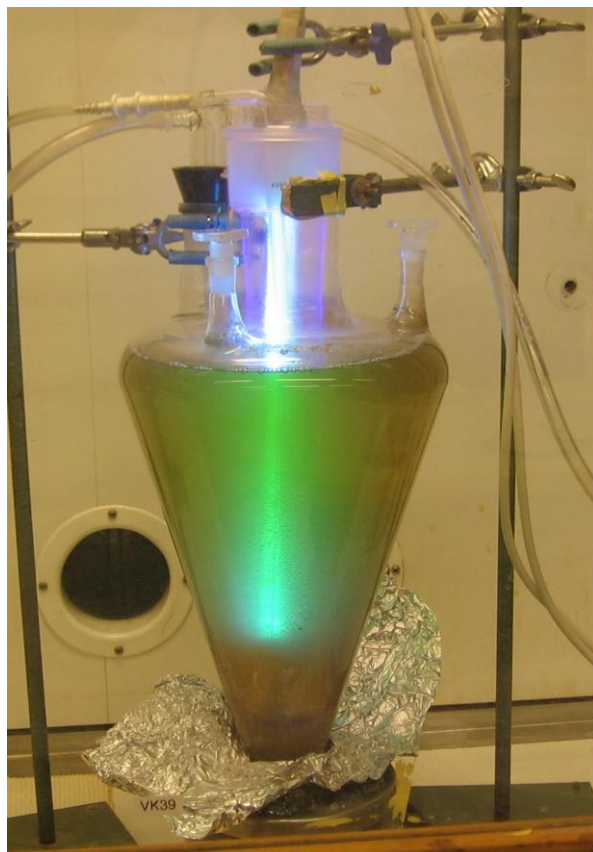
FIGURE 11. UV-reactor with UV-lamp on (Photo: Jukka Pohja 2011)
