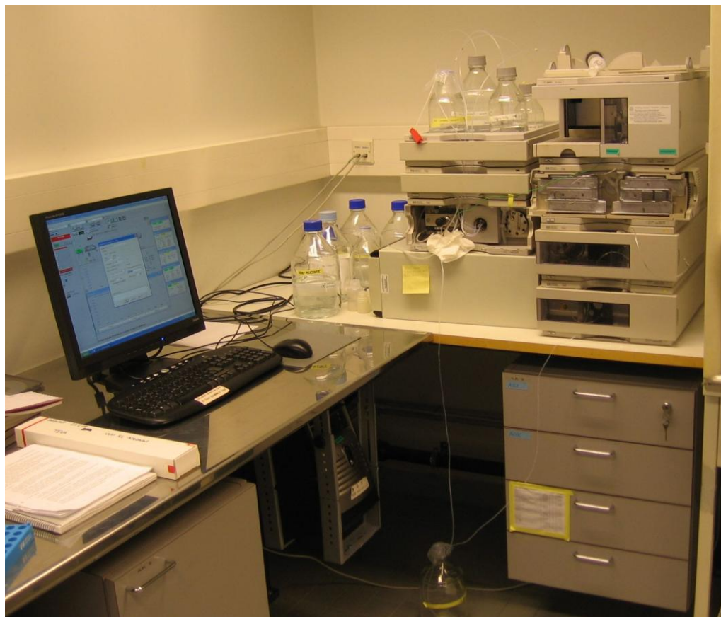
FIGURE 9. High Performance Liquid Chromatography system used (Photo: Jukka Pohja 2011)
