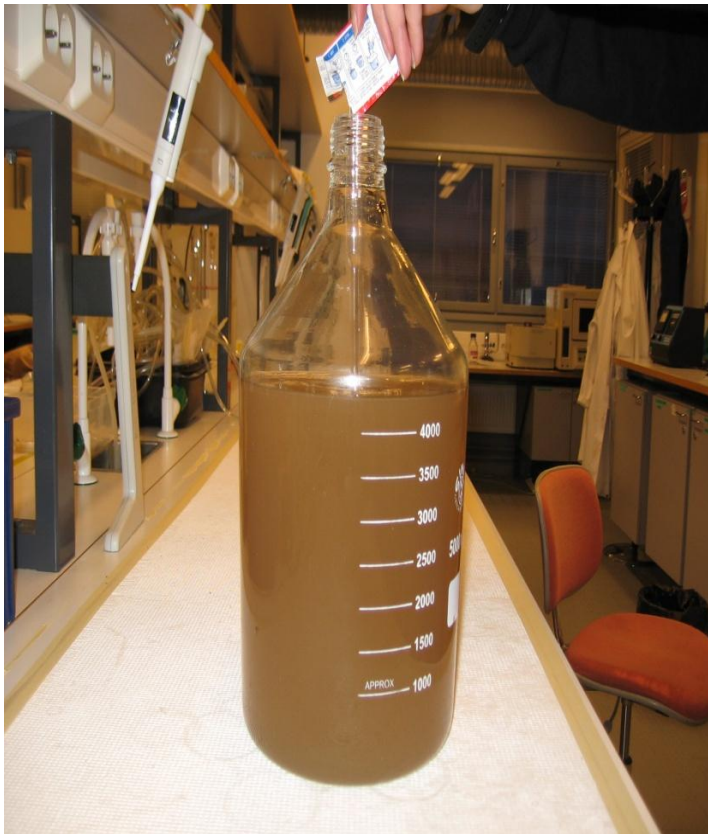
FIGURE 14. Adding of the coagulant powder (Photo: Jukka Pohja 2011)
