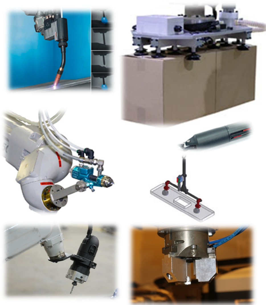
Figure 8 End-effectors (from top left clockwise) welding gun (End-Effectors, 2011), vacuum cup (End-Effectors, 2011), cutting tool (End-Effectors, 2011), magnet (Magnet type end effector, 2011), gripper, drill (End Effectors, 2011), and spray gun (End-Effectors, 2011)
