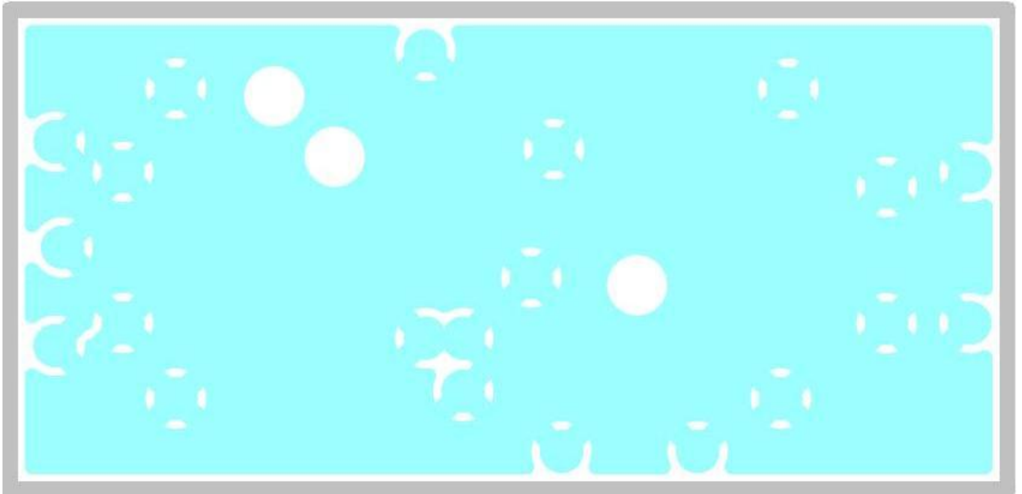
STURM2 amplifier board inner layer 2, GND
