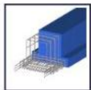
Inverted tee beam - automated reinforcement layout (52)
