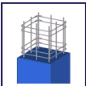
Columns - automated reinforcement layout (57)
