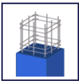
Columns - automated reinforcement layout (57)
