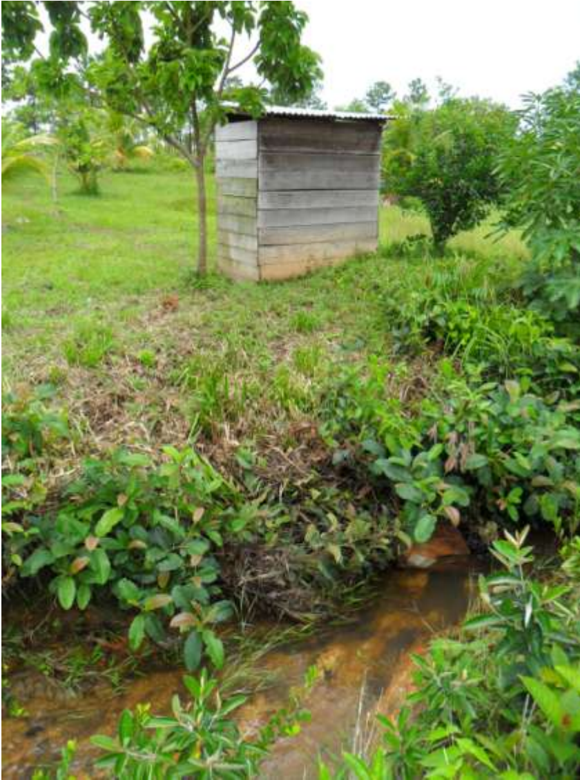
Pic 12 A poorly placed toilet. The toilet constructed above is too close to the stream. (Pietilä 2011)
