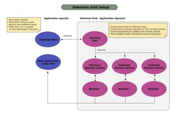
FIGURE 8. Selenium Grid Setup (Selenium Grid 2012).
