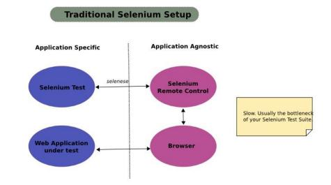
FIGURE 7. Normal Selenium Setup (Selenium Grid 2012).
