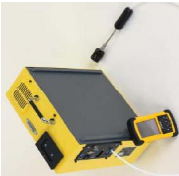
Figur 3. FTIR-analysator DX403 (Gasmot technologies Oy).
