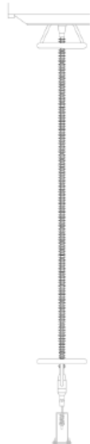
Picture 4. Signal column of a 735 kV FSC.
