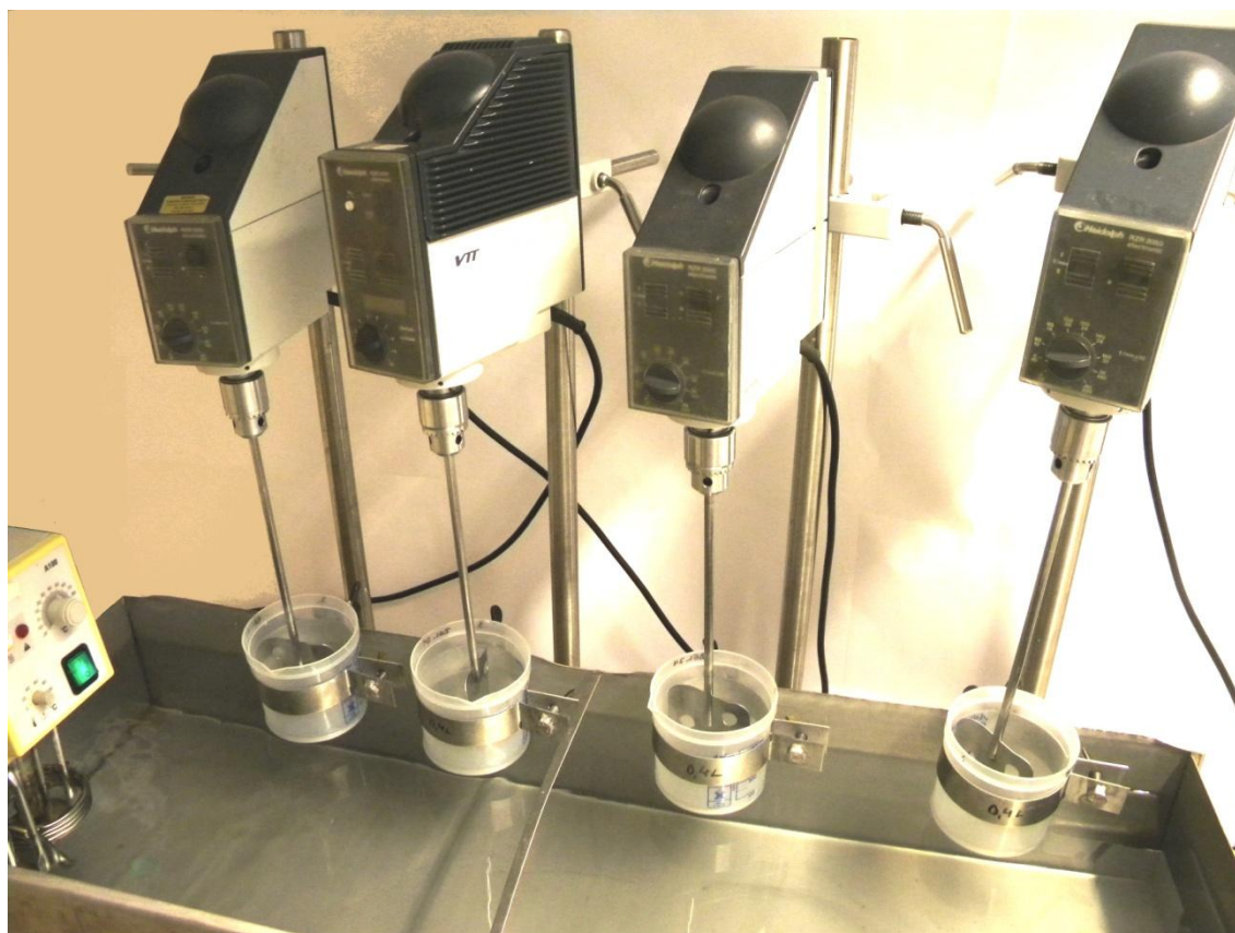
Figure 9. The set up for four parallel enzymatic hydrolysis bowls in a water bath supplied with drilling machine -type mixers.
