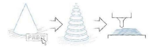
Figure 13. Stages of 3D printing (Nadarajah 2018)
