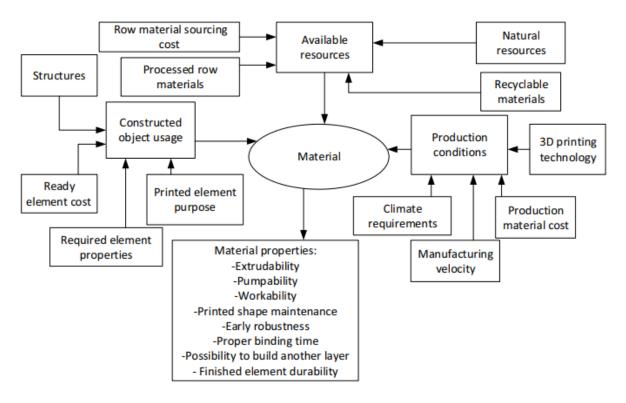
Figure 10. Building material composition for 3D printing and properties requirements (Pacewicz et al. 2018)
