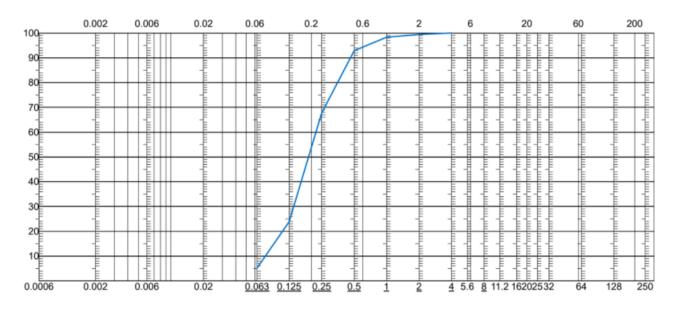
Figure 12. Sand particles distribution curve
