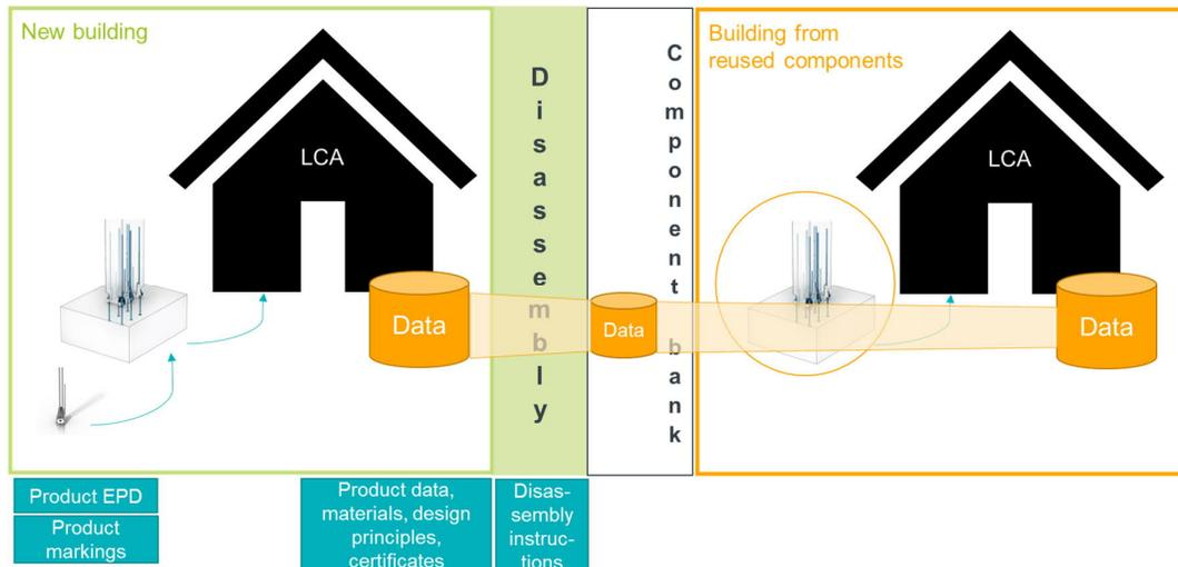
Figure 5. The data flow in the building process when reuse is included in the Peikko point of view.
