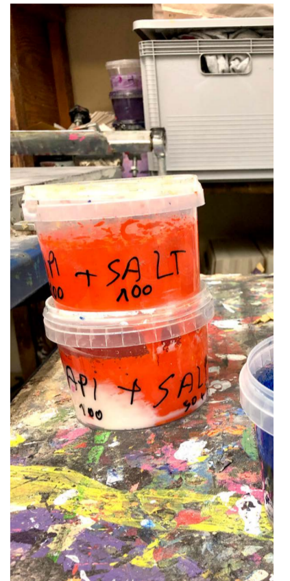
PICTURE 17. One of the tested ingredients for conductive ink was salt. (Kurki 2020)
