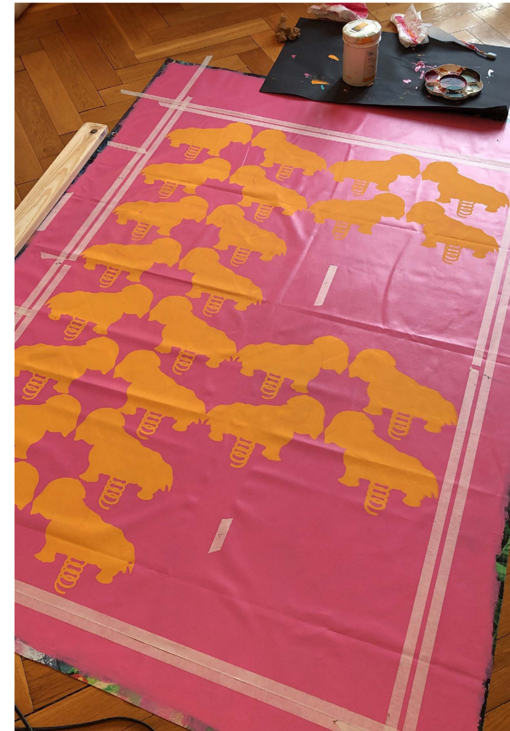
PICTURE 47. In silk screen printing, each color needs its own layer. (Kurki 2020)
