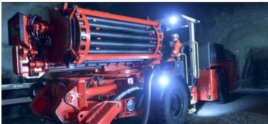
Figure 2. Longhole drill rig (Sandvik, 2020)
