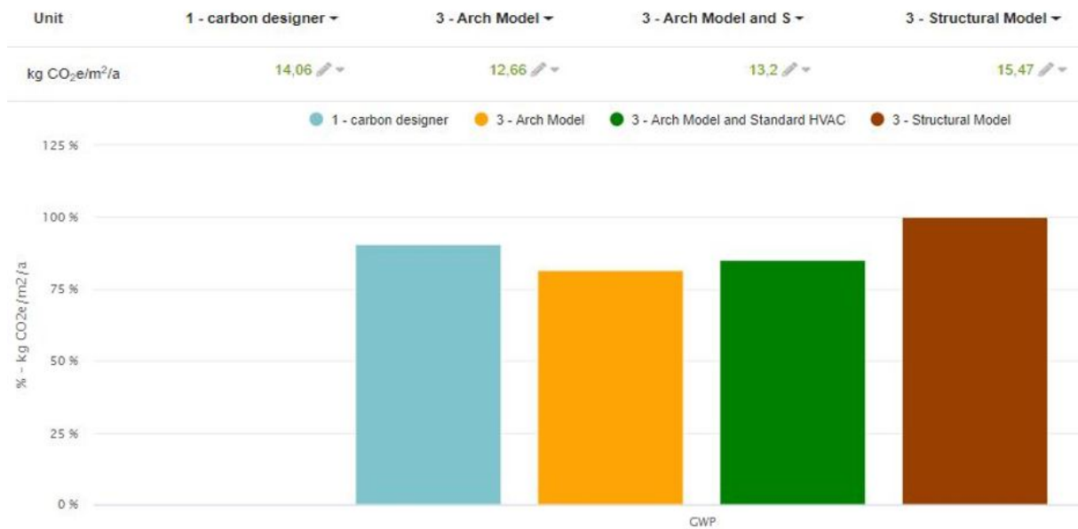
Figure 55: Third case study comparison of different design models final carbon emission results.
