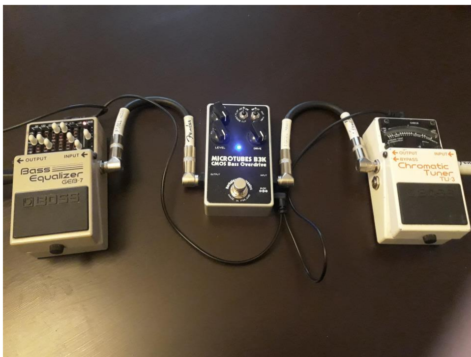
PICTURE 8. Bass connected to the chromatic tuner, to the Darkglass Bass Overdrive pedal and finally into the Bass Equaliser.
