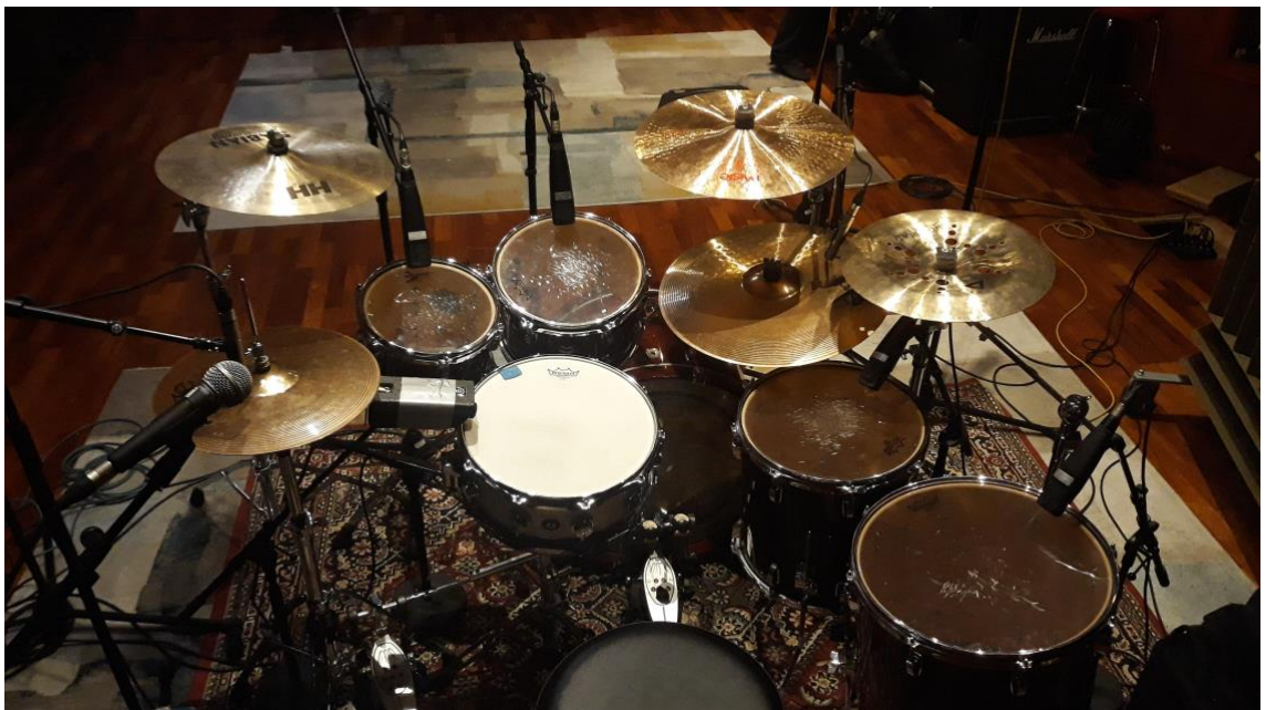
PICTURE 7. The drum set used and the microphone positions of the snare and toms.
