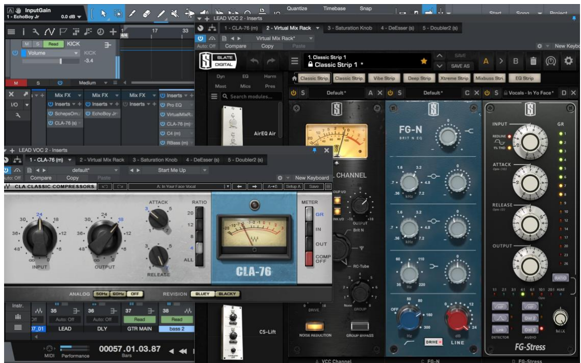
PICTURE 11. The compressor-chain. Note the significant high-end boost in the FG-N EQ, which is necessary for dark character of the SM-7b.
