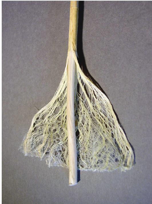
Picture 1. Image of hemp stalk with distinctly divided central woody core and loosened bast fibers (Sources: Natrij 2002 (Wikipedia))
