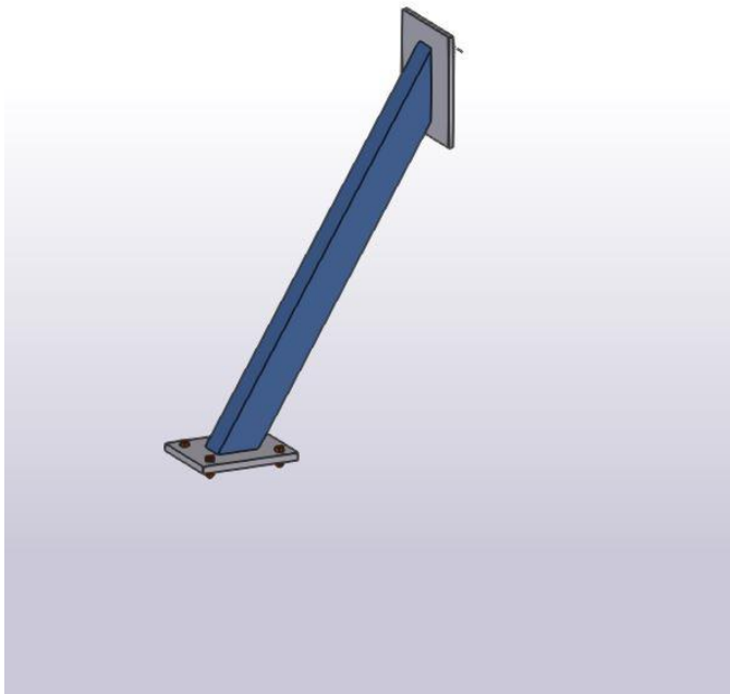
Figure 12. Bracing member of reaction frame.
