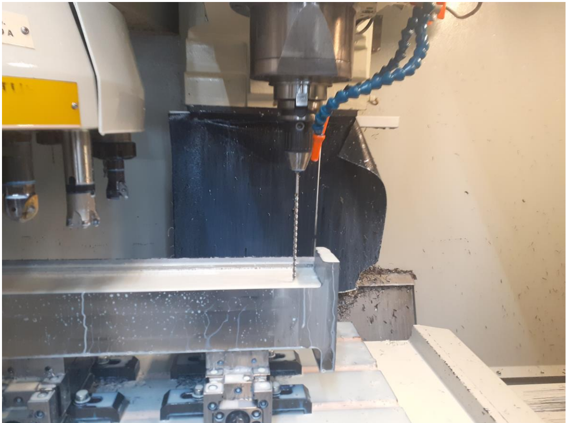
Photo 15. Internal oil channels required long drills. (Roni Ampuja 2021)
