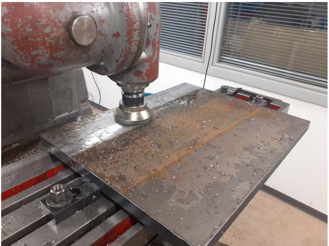
Photo 12. Base plate had to be done by manual mill since big enough CNC was not available. (Roni Ampuja 2021)
