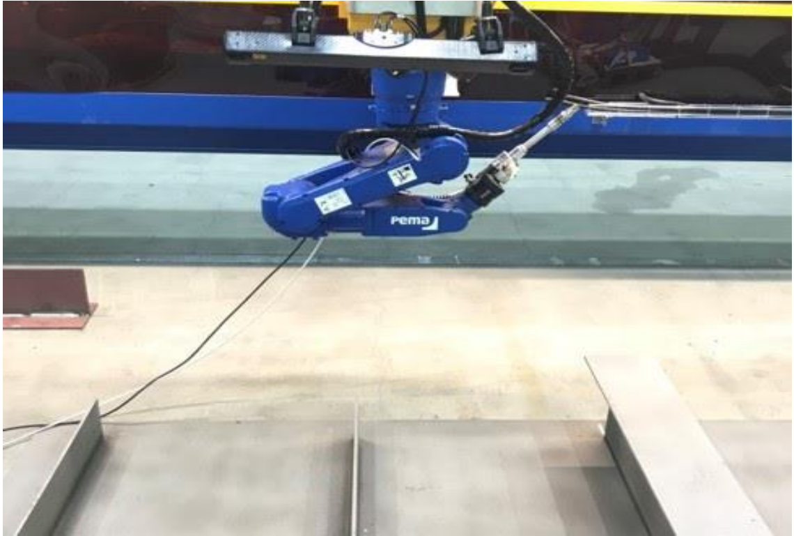
Figure 1. Scanner at 45 degrees relative to the ground
