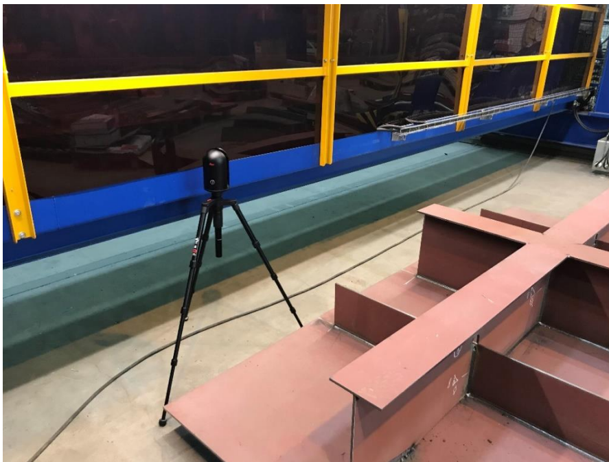
Figure 6. Scanning positioning of BLK360
