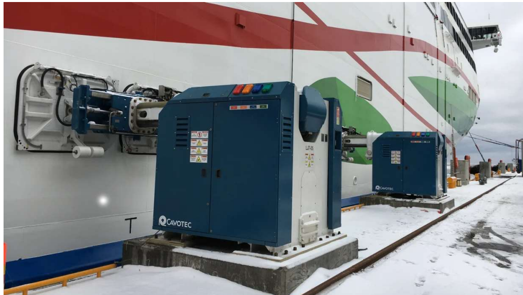
Figure 1. Vacuum automated mooring application in use, Megastar (owned by AS Tallink Grupp) alongside in Helsinki West Harbour, Terminal 2. (Cavotec, 2018)
