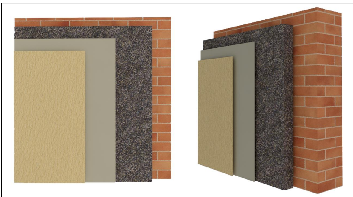
Fig. 28: ArchiCAD rendered model of the external multi-layered wall. Source: (By Author)
