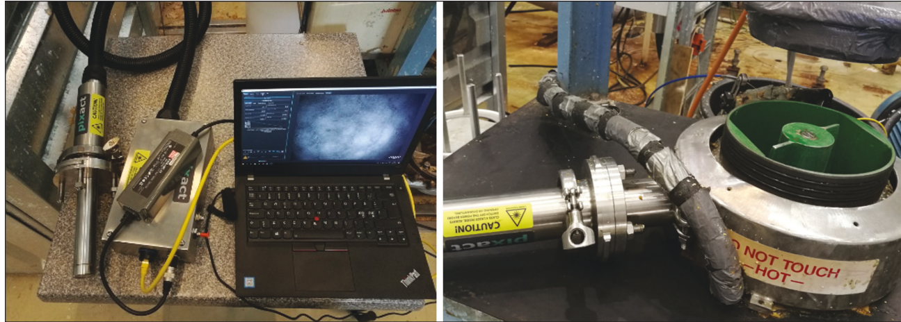
1. Compact bubble size measurement system connected to the Mark IV Quantum mixer/reactor [2].
