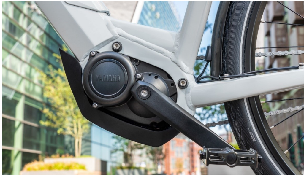
Figure 3. Mid-drive unit (YAMAHA e-bike, 2021)
