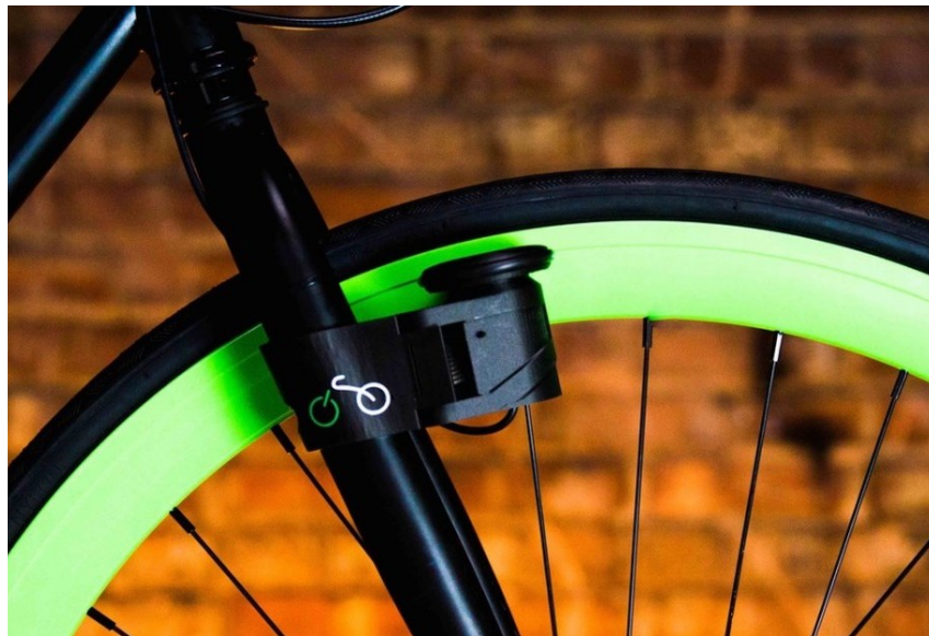
Figure 6. Dynamo attached on a bicycle (Pedalcell, n.d.)
