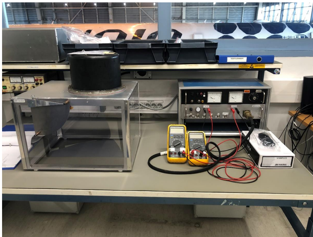
Figure 17: Landing light test jig on the left with landing light unit set on top, power supply and measuring equipment on the right
