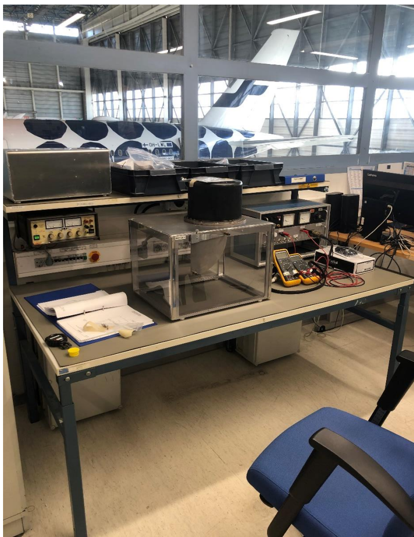
Figure 16: Test bench for the external lights
