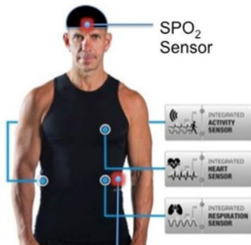
Figure 14. The Astroskin garment. A shirt originally developed for astronauts (Toscano et al., 2017, p. 7)
