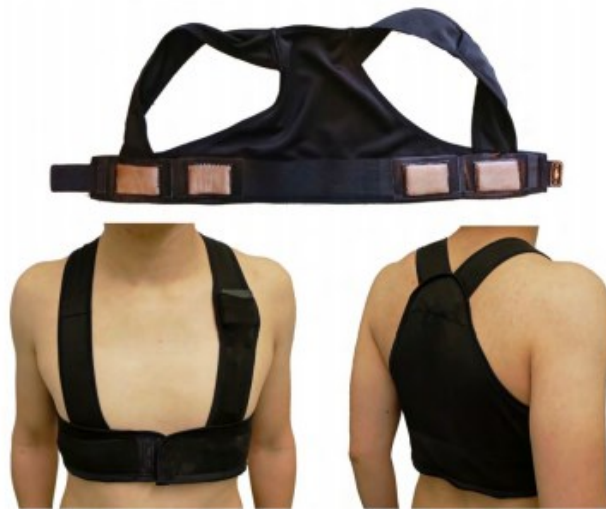
Figure 10. The smart vest includes four textile electrodes, that are used for measuring electrocardiogram (ECG) and thoracic electrical bio-impedance (TEB) (Yang et al., 2018, p. 3)
