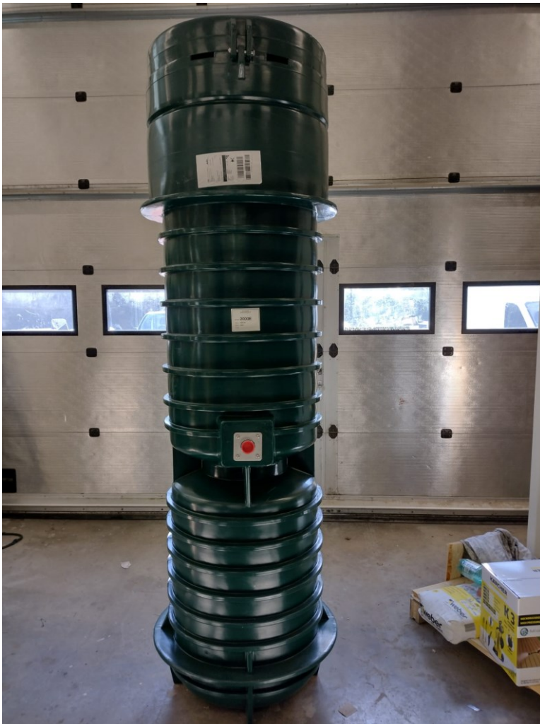
Figur 5. Pumphus LPS 2000E (Foto: Jimmy Englund, 2021)
