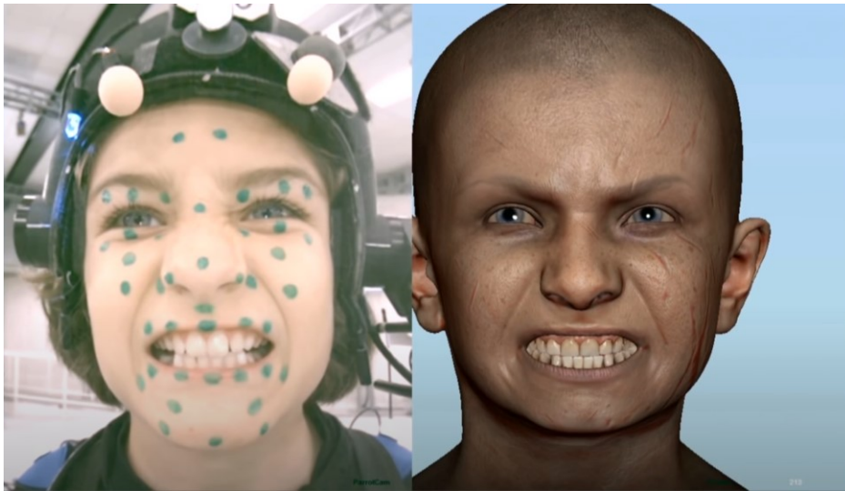
FIGURE 10. Motion capture data controlling a facial rig (Pinto & Grossman 2018).
