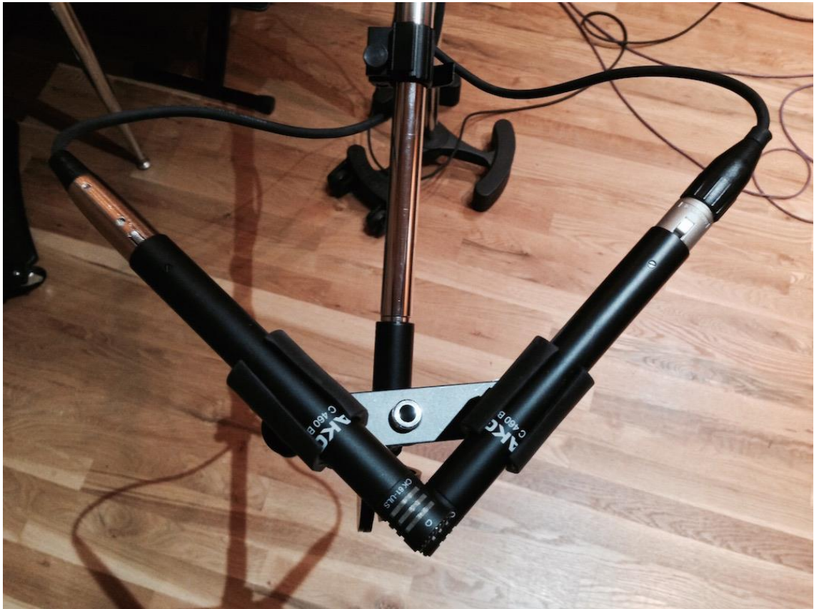
PICTURE 2. X/Y stereo miking technique (Sound Training College 2017)
