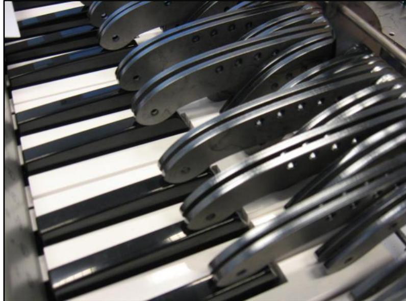
Figure 4 – Photo of a portion of the keys. In this image the fingers are not yet connected to the cables and the pull-up rubber bands are missing as well. (Photo: Artemis Project 2008)
