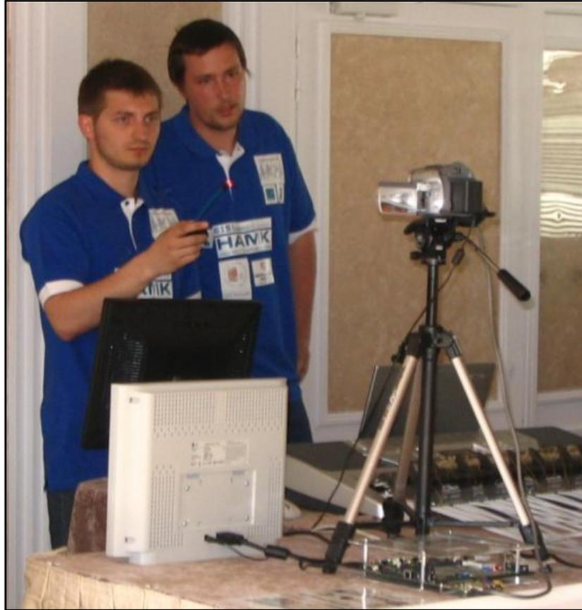
Figure 2 – *Tempo recognition unit in use at the Artemis competition. The tempo recognition units FPGA board is in the lower right corner of the image. Above the FPGA board is the camera. (Photo: Artemis Project 2008)*
