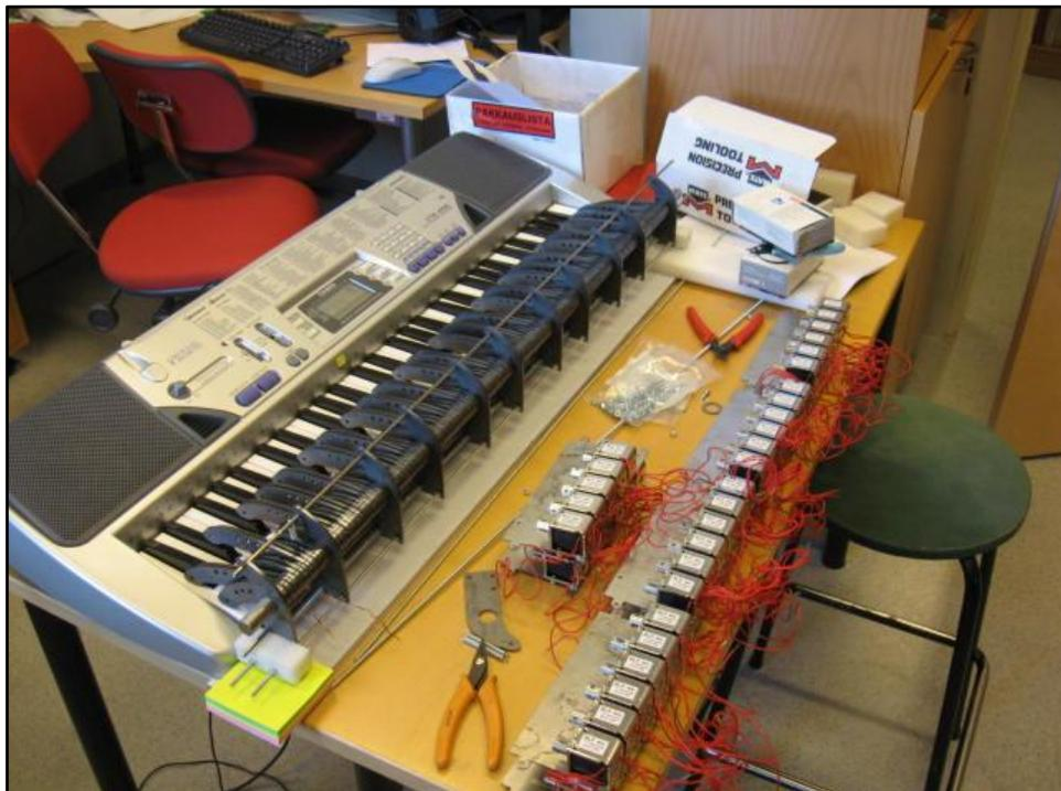
Figure 7 – Incomplete finger mechanics. There are 61 solenoids on the right side of the table. The solenoids were later put into acrylic frames with their respective mechanics controller boards. (Photo: Artemis Project 2008)
