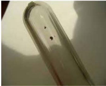
Picture 16 Contaminated RPET preform source: Large scale demonstration of the viability of Recycled PET (rPET) in Retail Packaging Coca-Cola Enterprises Ltd 2006
