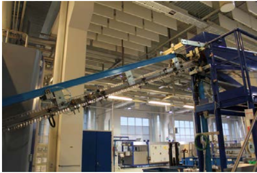
Picture 11 Preforms being transported into filling machine Picture Paul Fletcher 2011
