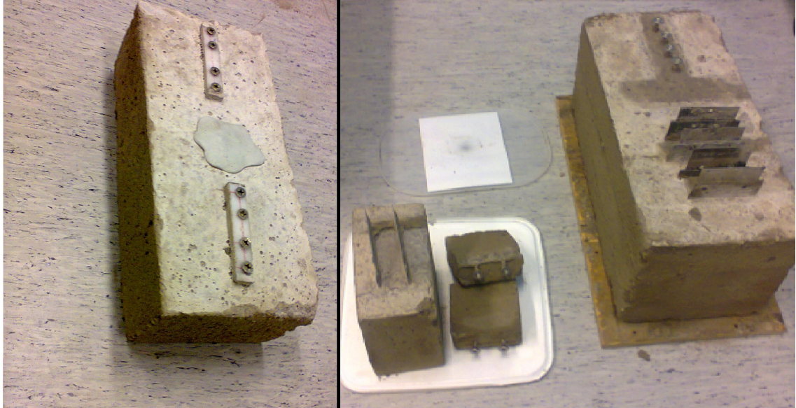
PICTURE 15. The test concrete objects and the sensors
