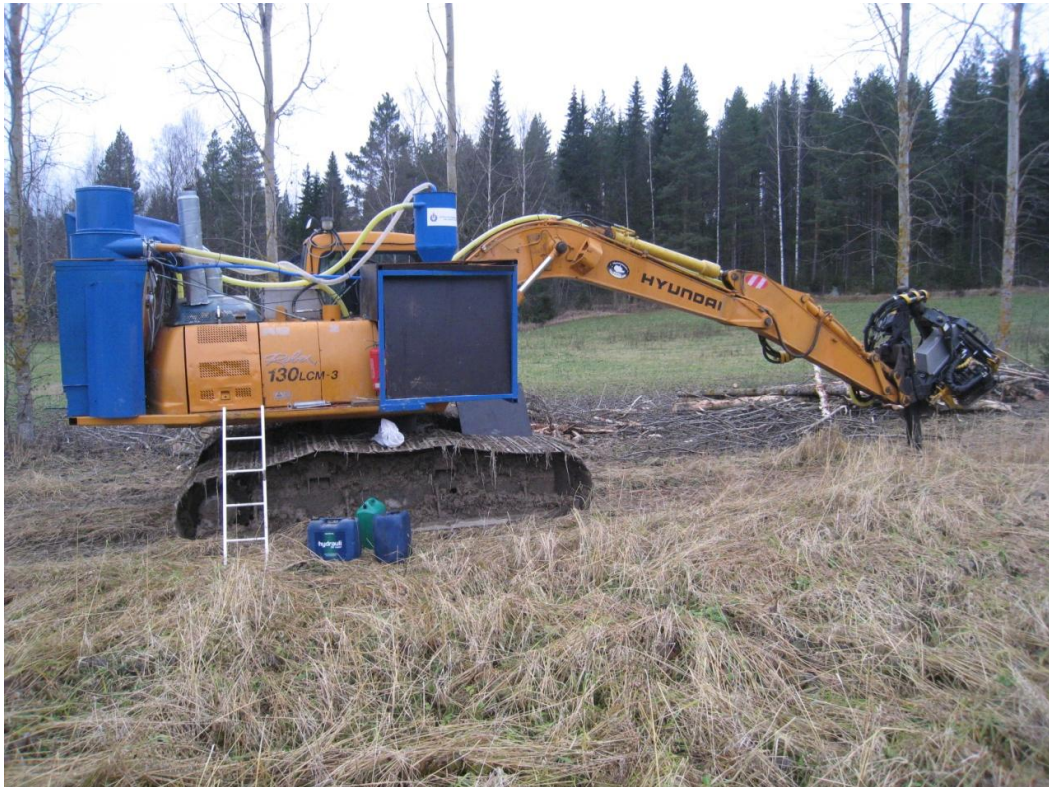
FIGURE 9. The prototype fitted on a digging machine transformed into a harvester.
