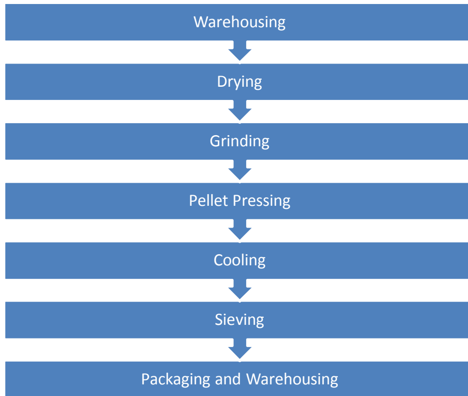
FIGURE 3. An example of a basic pellet pressing process. (Vapo 2009)
