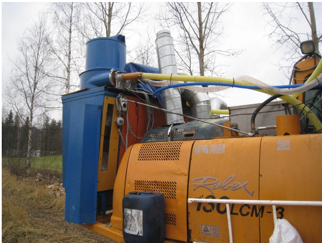
FIGURE 12. Sawdust goes through the pipes in to a drying system.
