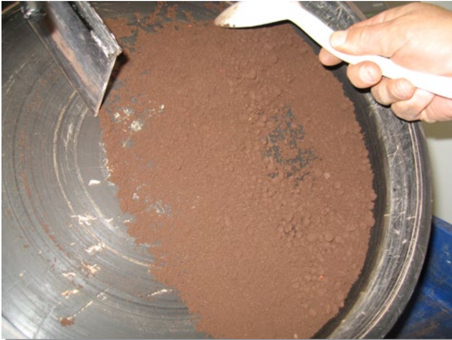
FIGURE 1. Product development work on by-product flows at the Environmental Laboratory of Mikkeli University of Applied Sciences – using a laboratory-scale granulation plate (photo by Hanne Soininen)
