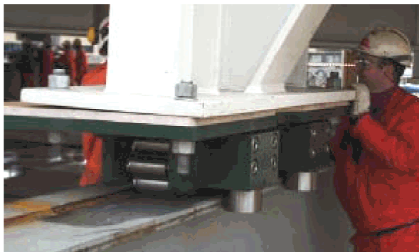
Figure 4.1.4: Hilman rollers equipped with guide rollers. /7/
