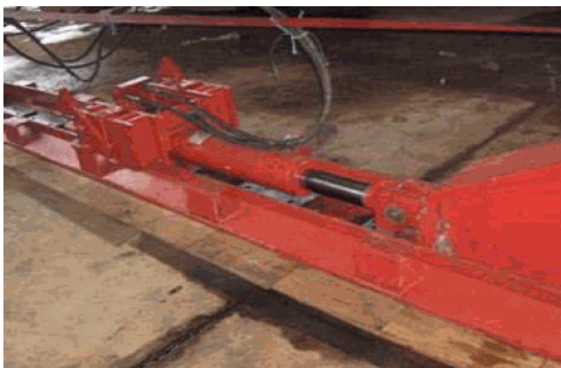
Figure 4.3.2: The push-pull unit. /13/
