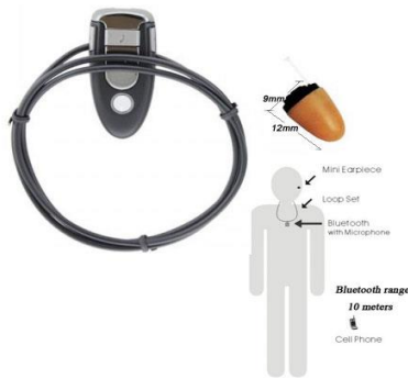
Figure 14: Induction loop system
