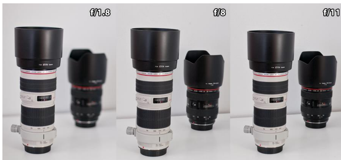
Figure 7. The effect of stopping down lens aperture
