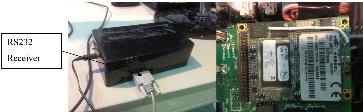
Figure 12. Wireless Sender Connected with PC and Wireless Receiver on Robot
