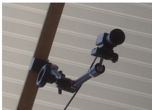
Figure 9. a High Speed Camera Connected to the Vision Server
