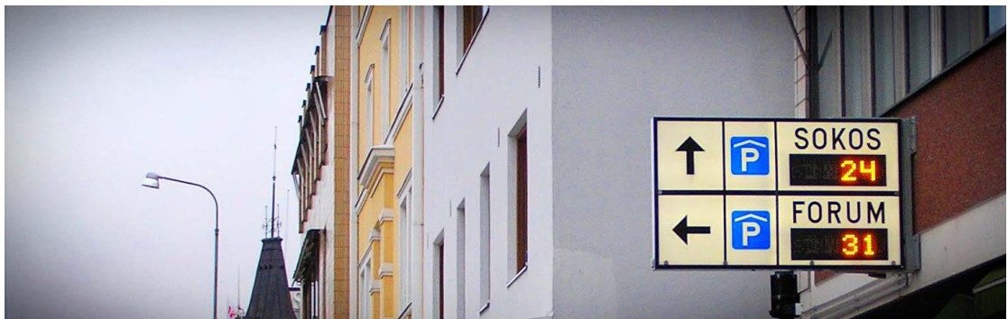
Figure 3 VMS's (Variable Message Signs) installed by the street. The sign displays available parking lots in two separate parking halls
