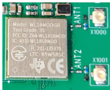
Figure 5: Orientation of wi-fi module on the panel PCB
