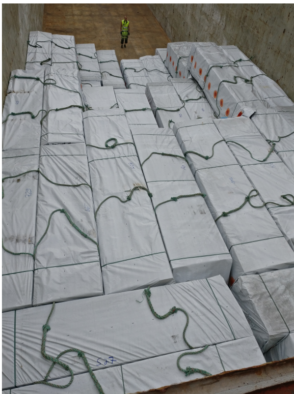
Figure 5. The cargo is loaded in layers of three until the midship section. (Björk, 2020).
