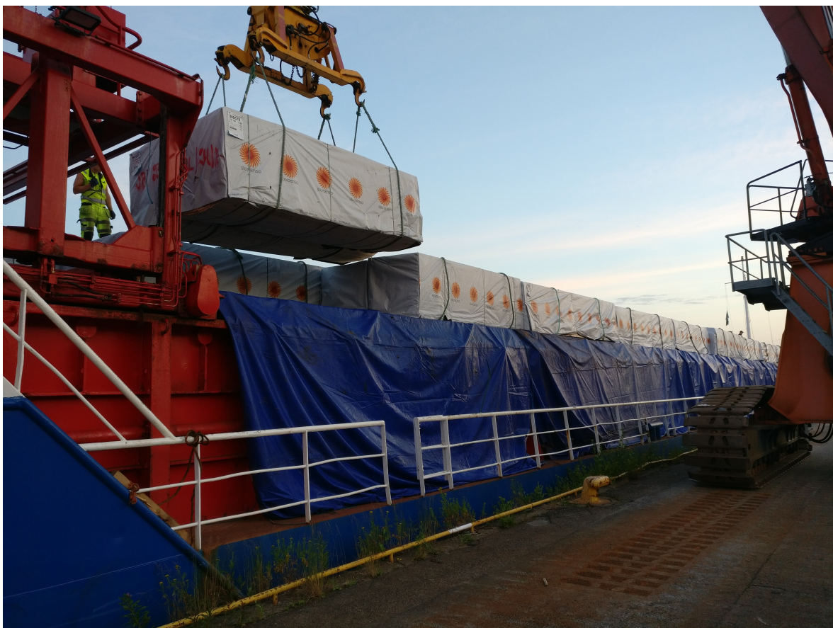
Figure 6. Tarpaulins were placed under the cargo and folded over after completion. (Björk, 2020).
