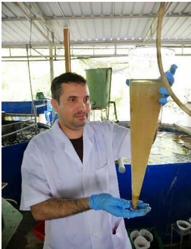
PICTURE 2. Conical beaker used to measure the growth of Biofloc (Beijnen and Yan 2019)
