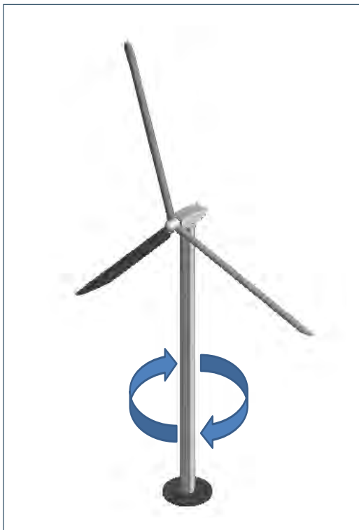
Figure 3.22 Power output control using an alignment to the wind, a yaw control.
