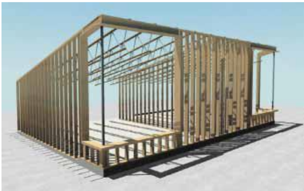
Figure 7: Typical wooden modular frame of classroom 134
