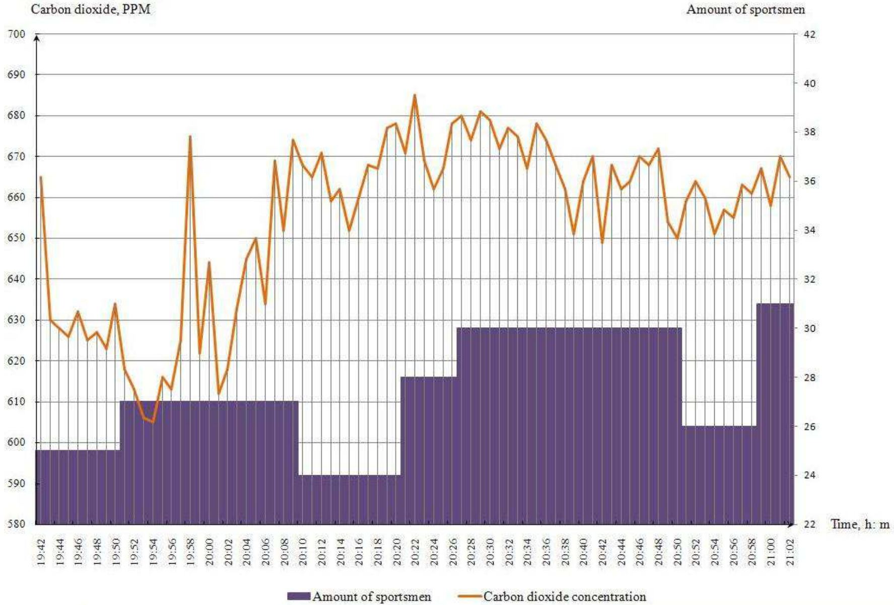
FIGURE 34. The monitoring of carbon dioxide concentration in air supported structure
