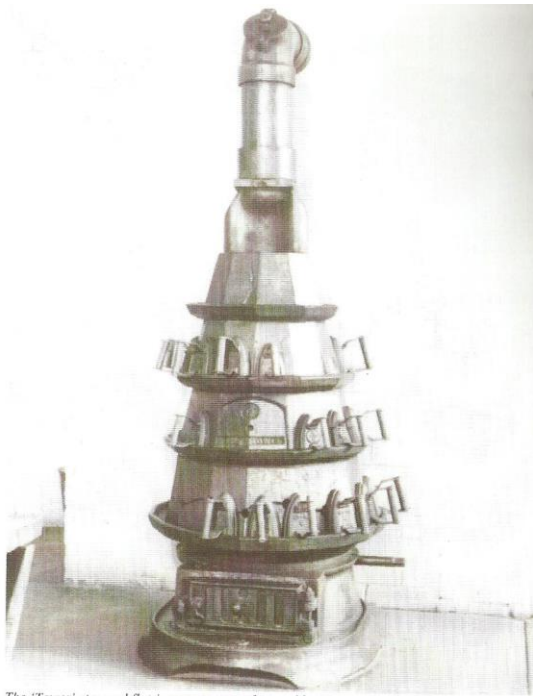
The 'Tower' stored flat-iron stove, manufactured by Thomas Readford & Co., London.
