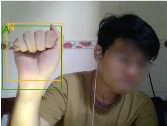
Figure 9 (3). The model got confused between letter A and N, because of the detailed background
